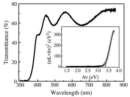
Fig. 3. Optical transmittance of the BZN film prepared on a MgO substrate. The relation  $(\alpha L * hv)^2$  versus  $h\nu$  is shown in the inset.
