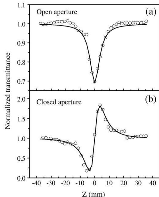
Fig. 4. Normalized (a) open-aperture and (b) closed-aperture Z-scan data of the BZN film. The solid lines indicate the theoretical fit.
