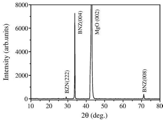
Fig. 1. XRD pattern of the BZN film on a MgO(001) substrate.
