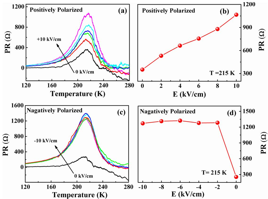
Fig. 4: (Color online) The temperature dependence of photoinduced resistance (PR, where  $PR = R_{\text{light}} - R_{\text{dark}}$ ) changes for the LSMO film by applying different electric fields to the LSMO/PMN-PT structure when PMN-PT is in (a)  $P_r^+$  and (c)  $P_r^-$  states, respectively. The field dependence of PR for the LSMO film measured at 215 K when PMN-PT is in (b)  $P_r^+$  and (d)  $P_r^-$  states, respectively.
