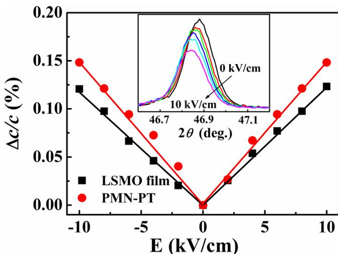
Fig. 5: (Color online) The relative changes in the pseudocubic lattice constants  $\Delta c/c$  of the LSMO film and the PMN-PT substrate as a function of electric field  $E$  from  $-10$  kV/cm to  $+10$  kV/cm. The inset shows the *in situ* XRD patterns in the vicinity of pseudocubic (002) reflection for the LSMO film under different electric fields.
