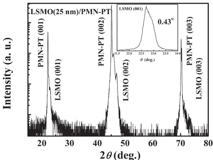
Fig. 1: X-ray diffraction (XRD) spectra of single-phase LSMO films grown on PMN-PT. The inset shows the rocking curve of the (002) reflection of LSMO.
