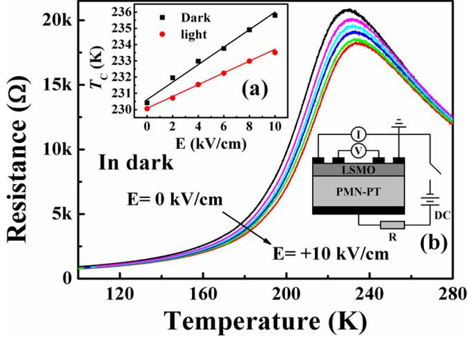
Fig. 3: (Color online) The temperature dependence of resistance for the LSMO film by applying an electric field  $E$  from 0 to 10 kV/cm on the LSMO/PMN-PT structure when PMN-PT was in  $P_r^+$  state and measured kept in the dark. The inset (a) shows  $T_c$  vs.  $E$  when LSMO is kept in the dark and under the irradiation of 532 nm laser, respectively. The inset (b) presents the schematic diagram of the LSMO/PMN-PT structure and the measurement circuit.
