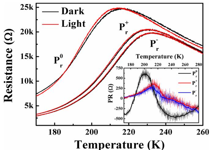
Fig. 2: (Color online) The temperature dependence of resistance for the LSMO film kept in the dark and under the irradiation of 532 nm laser when PMN-PT was in  $P_r^0$ ,  $P_r^+$ , and  $P_r^-$  states, respectively. The inset shows the PR changes of the LSMO film with temperature when PMN-PT was in  $P_r^0$ ,  $P_r^+$ , and  $P_r^-$  states, respectively.
