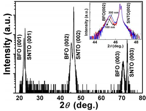
Fig. 1: (Color online) XRD diffraction pattern for the 100 nm BFO thin film. The inset shows the expanded area of (002) peaks from both films and substrates, indicating the effect of the epitaxial strain on the BFO films with different film thicknesses.
