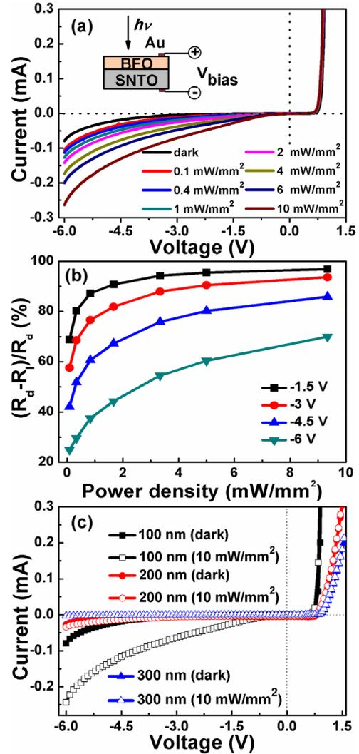
Fig. 2: (Color online) (a)  $I$ - $V$  curves measured on a 100 nm BFO thin film in the dark and under the irradiation of a 325 nm laser. The inset shows the schematic circuit of measurement. (b) The photo-resistance of sample S1 changes with the power density of the laser at different reverse bias values. (c) Variation of  $I$ - $V$  curves of samples S1, S2, S3 measured in the dark (solid symbols) and under the irradiation (open symbols) of a 325 nm laser.
