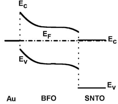
Fig. 4: Schematic band structure for the Au/BFO/SNTO structure at thermal equilibrium.
