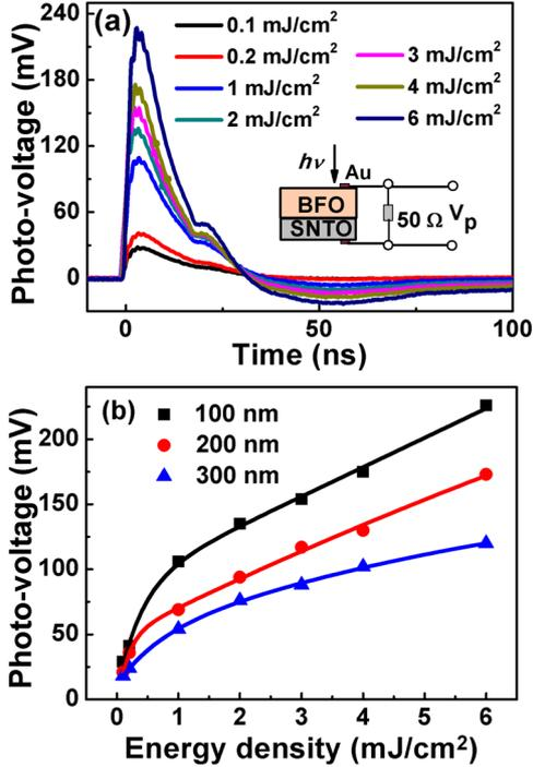
Fig. 3: (Color online) (a) Variation of photo-voltages of sample S1 with different energy density under the excitation of a pulsed Nd:YAG laser. The inset displays the schematic circuit of measurement. (b) The photo-voltages of samples S1, S2, S3 under the excitation of a pulsed Nd:YAG laser.
