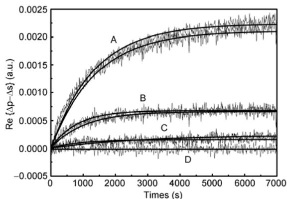
**Figure 3** The variations of OIRD  $\text{Re}\{\Delta_p-\Delta_s\}$  signal with time. Curves A, B, C and D correspond to different concentrations of IgG, 1 mg/mL, 0.5 mg/mL, 0.25 mg/mL and 0 mg/mL (from the slide surface without mouse IgG), respectively.
