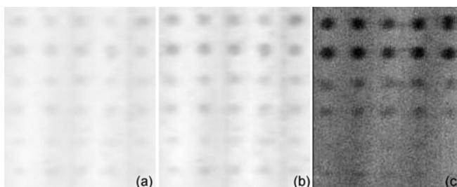
**Figure 2** The two dimensional scanning images of OIRD  $\text{Re}\{\Delta_p-\Delta_s\}$  intensity signals. (a) Before reaction; (b) after reaction; (c) the differential image of OIRD  $\text{Re}\{\Delta_p-\Delta_s\}$  signal obtained by subtracting Figure 2(a) from Figure 2(b).
