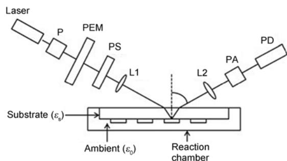
**Figure 1** The schematic diagram of OIRD setup for the label-free and real-time detection of IgG protein microarray. Laser, a 7 mW He-Ne laser; P, polarizer; PEM, photoelastic modulator; PS, 1/2 plate; L1 and L2, lens; PA, polarization analyzer; PD, photodiode detector.
