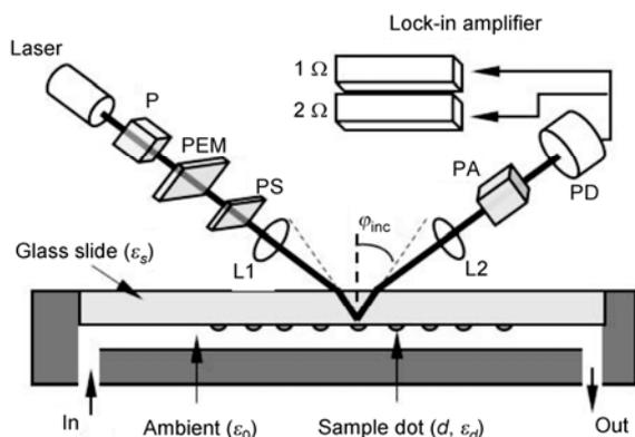
**Figure 1** Schematic diagram of OIRD system for label-free, high-throughput and real-time detection of biomolecules interactions. Laser: a 17 mW He-Ne laser; P: polarizer; PEM: photo elastic modulator; PS: phase shifter ( $1/2$  plate); L1 and L2: lens; PA: polarization analyzer; PD: photodiode detector.
