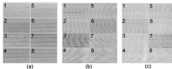
**Figure 4** 2D images of OIRD of the protein microarray including 10080 sample dots. (a) Before reaction of the microarray. (b) 2D differential images of OIRD after and before reaction between the protein microarray with Goat Anti-mouse IgG of mg/mL. (c) 2D differential images of OIRD after and before reaction between the protein microarray with Goat Anti-rabbit IgG of mg/mL.
