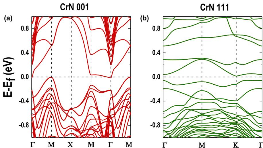
FIG. 4. Orientation-dependent band structure of CrN films. (a), (b) Band structures of CrN films with the fixed thickness of 10 u.c. The band gap in CrN 001 films is  $-13$  meV, which suggests a metallic state. In contrast, the band gap in CrN 111 films with an identical thickness is  $66$  meV, which demonstrates an insulating state.
