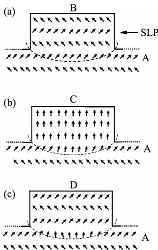
Fig.5 Cross sectional schematic illustration of the model related to the switching behavior for (a)  $I < I_{th1}$ ; (b)  $I_{th1} < I < I'_{th1}$ ; (c)  $I'_{th1} < I < I_{th2}$ .  $A$  is the “static” CAF state of the bottom electrode.  $B$ ,  $C$  and  $D$  denote the “free” magnetic states at  $I < I_{th1}$ ,  $I_{th1} < I < I'_{th1}$  and  $I'_{th1} < I < I_{th2}$ , respectively. The arcuate dashed line marks the boundary between the free and static regions
