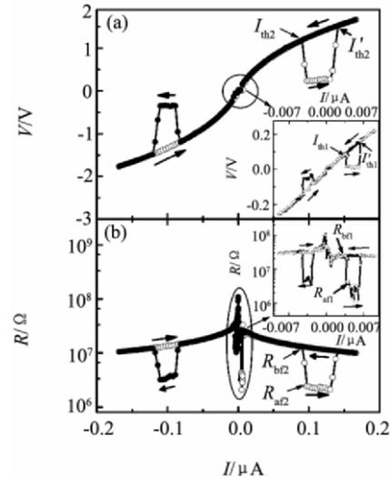
Fig.3  $V$ - $I$  characteristic (a) and the corresponding  $R$ - $I$  curves (b) of a 60 nm thick SLP at 120 K. The insets in (a) and (b) show the close view at low current.  $I_{th}$ s and  $I_{th}$ 's denote the threshold currents at the switchings,  $R_{bf}$ s and  $R_{af}$ s the resistances before and after the switching at  $I_{th}$ s
