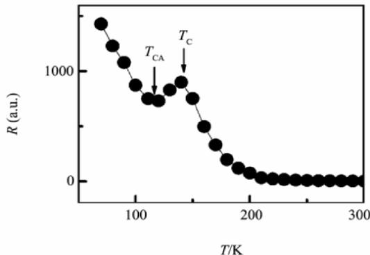
Fig.2 Temperature dependence of the resistance of an SLP
