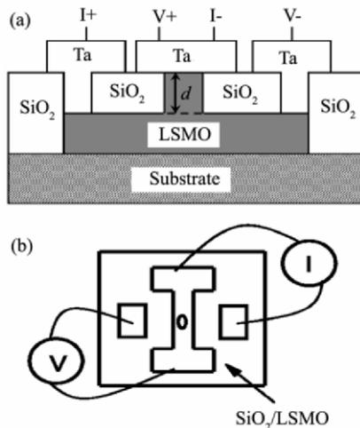
Fig.1 Cross sectional (a) and planar (b) views of the measuring circuit configuration.  $d$  denotes the thickness of SLP
