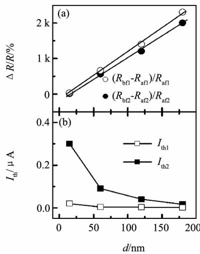
Fig.4  $\Delta R/R$  value (a) and the threshold current  $I_{th}$  (b) as a function of the SLP thickness  $d$
