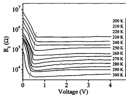
FIG. 5. The voltage dependence of junction conductive resistance at different temperature. The dotted line delineates the threshold voltage defined at that point the current obviously starts to increase.
