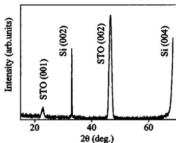
FIG. 2. XRD profile of the SrTiO<sub>3-δ</sub> film prepared on Si (100) substrate.
