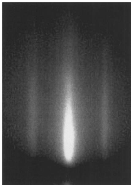
FIG. 1. RHEED pattern of the SrTiO<sub>3-δ</sub> film with a thickness of 150 Å on Si (100) substrate at 620 °C under 2 × 10<sup>-4</sup> Pa.
