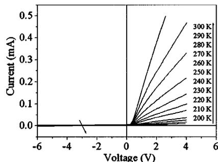
FIG. 4. The  $I$ - $V$  curves of SrTiO<sub>3-δ</sub>/Si junction in a wide temperature range of 200–300 K.
