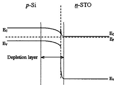
FIG. 6. Energy band diagram for SrTiO<sub>3-δ</sub>/Si junction.
