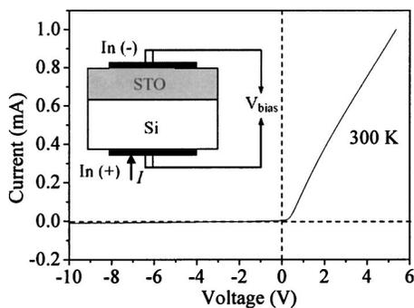
FIG. 3. The current-voltage ( $I$ - $V$ ) curve of SrTiO<sub>3-δ</sub>/Si junction measuring in a wide applied voltage scope at room temperature. The inset is the schematic structure of present  $p$ - $n$  junction.
