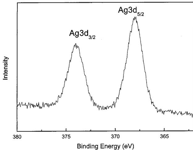
Fig. 3. X-ray photoelectron core-level-spectra of Ag 3d for the Ag:BaTiO<sub>3</sub> composite films.
