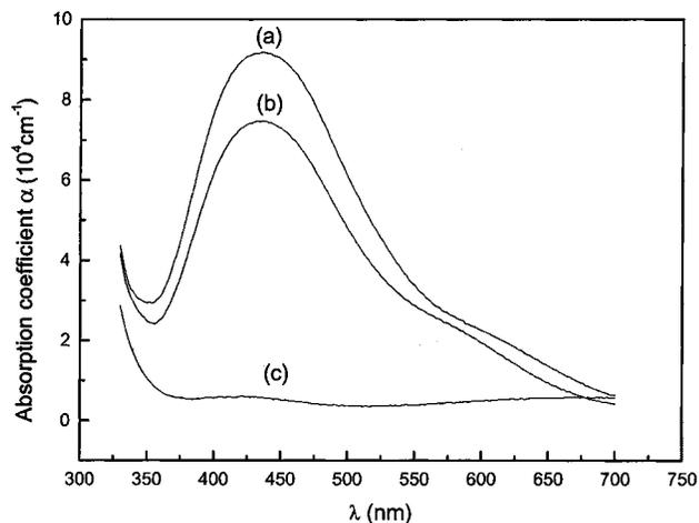
Fig. 4. Absorption spectra for sample A (without an applied electric field) and sample B (with an applied electric field of 1000 V/cm). Curve (c) is the absorption spectrum for the pure BaTiO<sub>3</sub> film.
