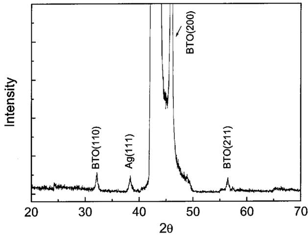
Fig. 2. X-ray diffraction patterns of Ag:BaTiO<sub>3</sub> composite films grown at 600°C on MgO substrates.
