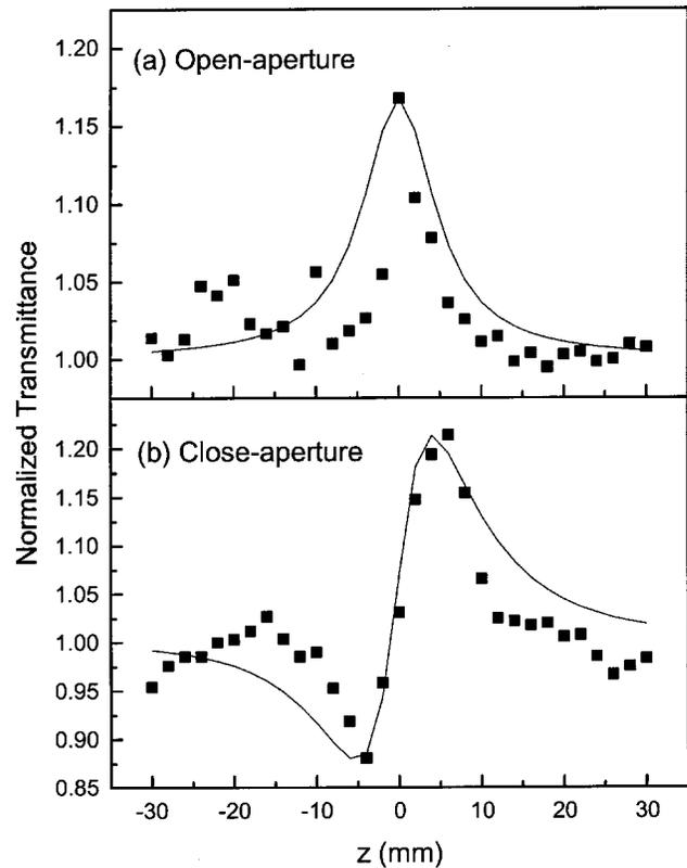
Fig. 5. The  $z$ -scan data of sample A (without an applied electric field) with (a) an open and (b) a closed aperture. The solid curves indicate the theoretical fit.
