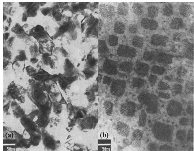
Fig. 1. TEM images of the Ag:BaTiO<sub>3</sub> composite films: (a), sample A (without an applied electric field); (b), sample B with an applied electric field of 1000 V/cm.
