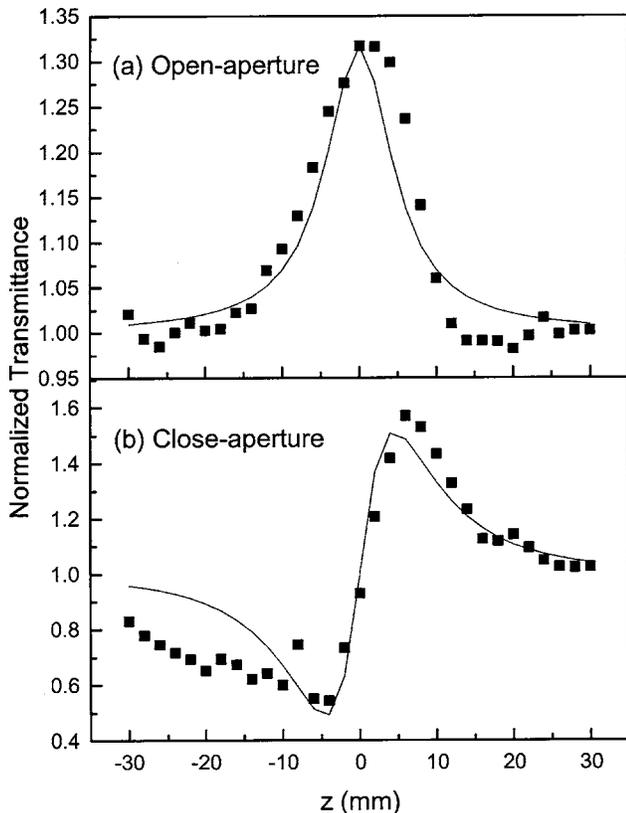
Fig. 6. The  $z$ -scan data of sample B (with an applied electric field of 1000 V/cm) with (a) an open and (b) a closed aperture. The solid curves indicate the theoretical fit.
