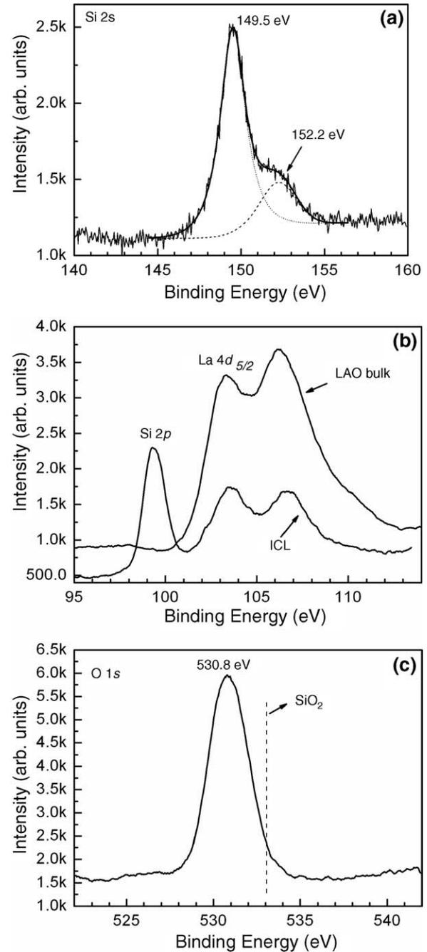
Fig. 3. XPS spectra for (a) Si 2s core level of the ICL on Si substrate, (b) La 4d core level of the ICL on Si substrate (bottom) and a clean bulk LAO (top), (c) O 1s core level of the ICL on Si substrate. The ICL sample was formed by the first step of the two-step approach.
