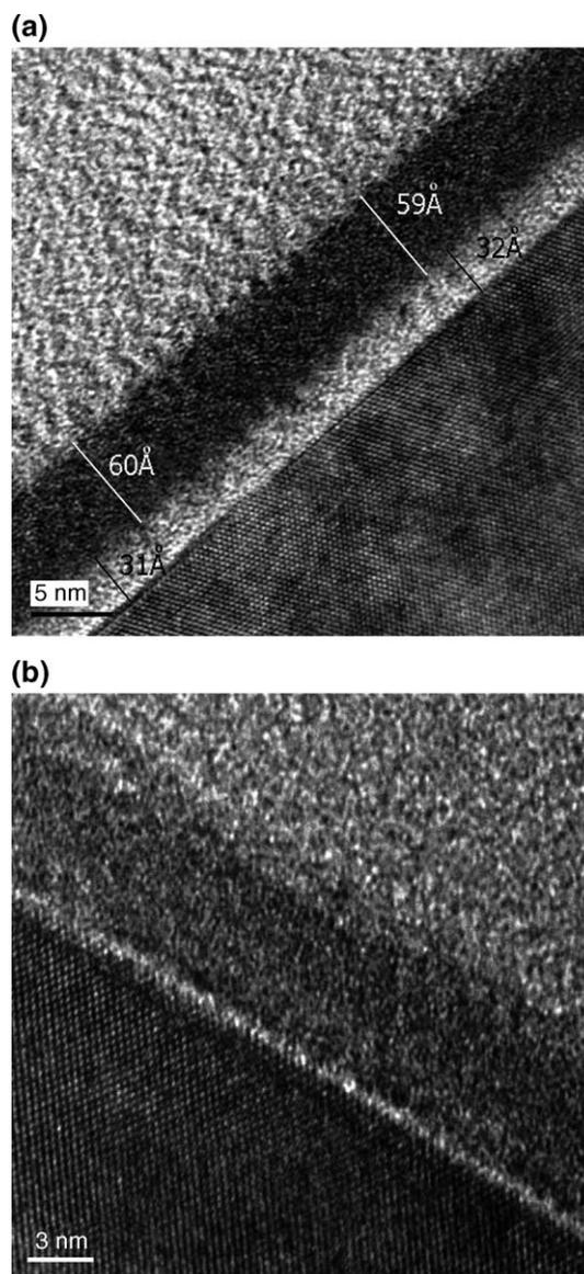
Fig. 1. HRTEM images of the LaAlO<sub>3</sub> layers: (a) directly deposited on Si substrate at the oxygen pressure of 0.2 Pa and substrate temperature of 700 °C; (b) deposited via the two-step approach.
