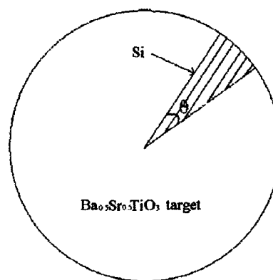
FIG. 1. Schematic configuration of the Si–BST target controlling the Si concentration in the thin film.
