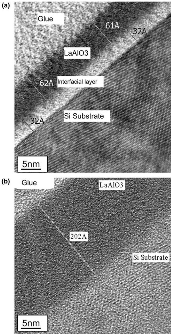
Fig. 1. HRTEM images of LAO films deposited in different oxygen pressure: (a) in 0.1 Pa at 700 °C; (b) in  $1 \times 10^{-4}$  Pa at 700 °C.
