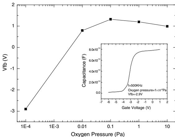
Fig. 3. Influence of oxygen pressure on the flatband voltages. The inset of the figure is the  $C-V$  curve of LAO films deposited in  $1 \times 10^{-4}$  Pa oxygen pressure.
