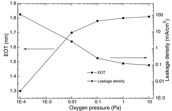
Fig. 2. Variations EOT and leakage current with the oxygen pressure during film fabrication.
