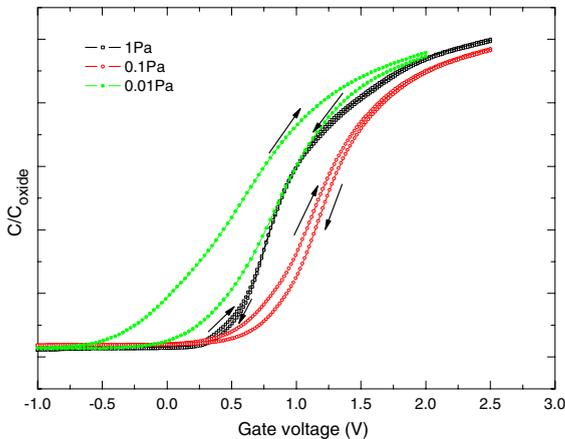
Fig. 4. Normalized  $C-V$  hysteresis loop characteristics of LAO films deposited in 0.01, 0.1 and 1 Pa oxygen pressures.
