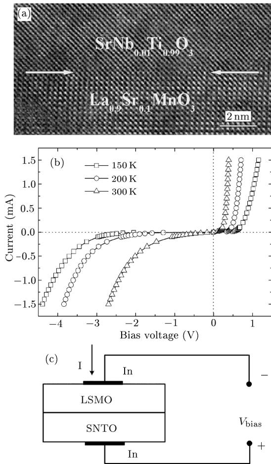
**Fig. 1.** (a) Cross-sectional HRTEM structural image of the interface in an LSMO/SNTO p-n junction; (b) the  $I$ - $V$  curves of the p-n junction at various temperatures; (c) the illustration of the p-n junction for electrical measurement.
