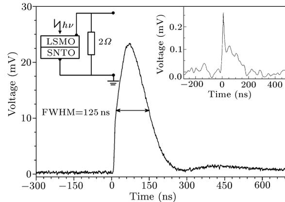
**Fig. 3.** Transient response of the photovoltage under the same condition as Fig. 2, except a  $2\Omega$  resistance connected in parallel across the p-n junction. Inset displays a schematic circuit of the sample measurement and the transient response of the photovoltage illuminated on the surface of the SNTO substrate of the p-n junction by a 308-nm laser pulse.
