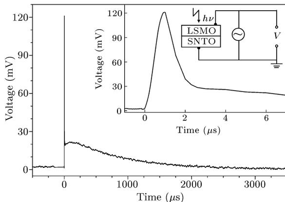
**Fig. 2.** Variation of the open-circuit photovoltage with time excited by a 308-nm excimer laser beam on the LSMO film of the p-n junction. The zoom of the sharp rise and the schematic circuit of the sample measurement are shown in the inset.
