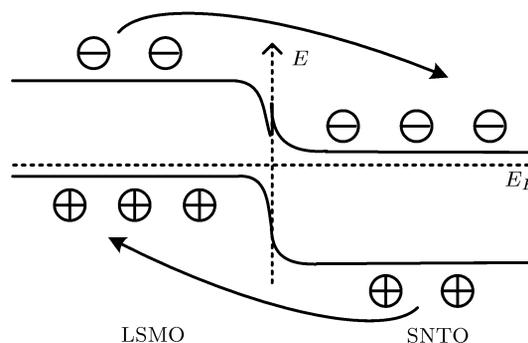
Fig. 5. Schematic band diagram of the LSMO/SNTNO p-n junction and the carrier movement induced by laser.
